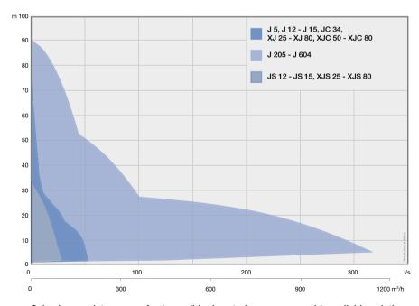
Sulzer's complete range of submersible dewatering pumps provides reliable solutions for all major dewatering needs.
