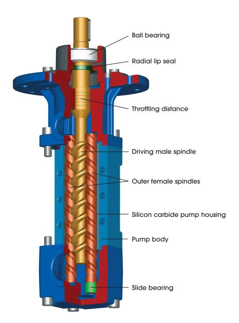
Silicon carbide spindle housings
