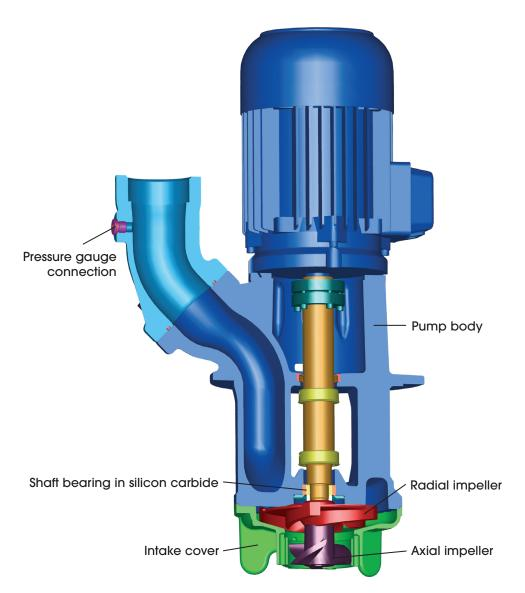
Quick suctioning immersion pumps equipped with the patented "BRINKMANN's Suction De-aeration System" are excellently suited to pumping extremely inflated fluids (emulsions resp. cooling/cutting oils) as they occur in heavy cutting when turning, milling or grinding. The quick suctioning immersion pumps reach stable working conditions as soon as the liquid level reaches the suction inlet.
