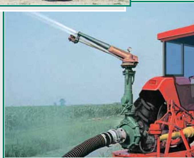
Applicazione al sollevatore del trattore Tractor hydraulic lift mounted pump outfit Emploi sur relevage du tracteur
