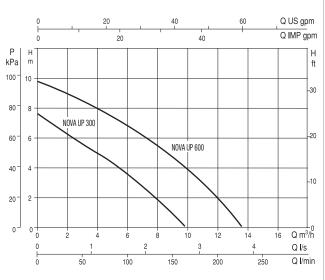
The performance curves are based on kinematic viscosity values = 1 mm<sup>2</sup>/s and density equal to 1000 kg/m<sup>3</sup>. Curve tolerance according to ISO 9906.
