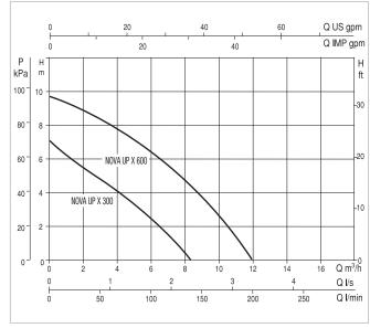
The performance curves are based on kinematic viscosity values = 1 mm²/s and density equal to  $1000 \text{ kg/m}^3$ . Curve tolerance according to ISO 9906.
