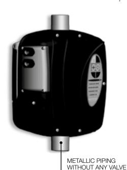
Electronic device based on inverter technology for electric pumps control. It controls the start-up and stop of the electric pump and modulates the motor rotations based on the water intake, maintaining a constant preset working pressure. It ensures high comfort for the end user, significant energy savings and longer life of the plant, typical advantages of inverter autoclave systems, including dry running protection for the electric pump
