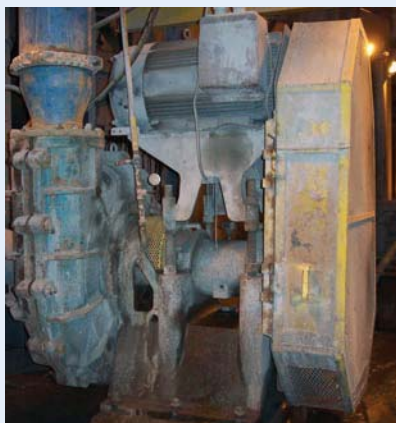
SRL-XT 14x12-36 on Ball Mill Discharge Service
