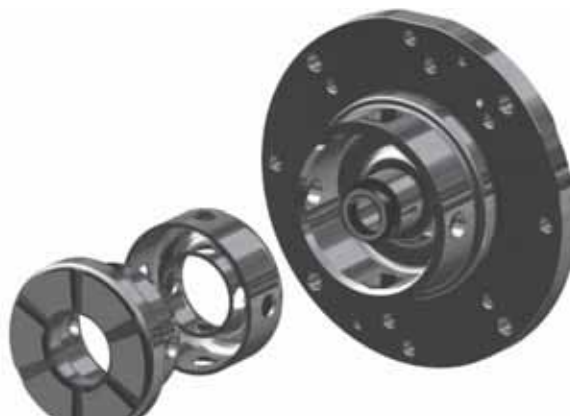
Fig. 11 Removing the thrust bearing and support
