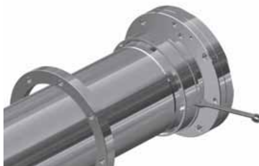
Fig. 27 Separating the pump and sleeve
