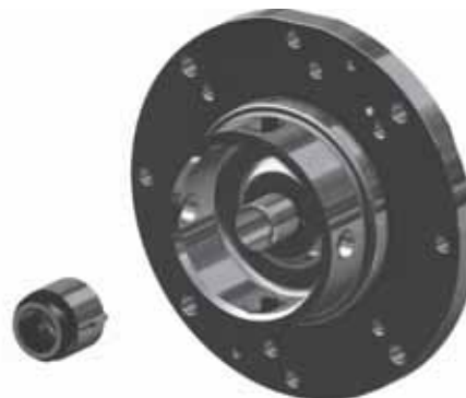
Fig. 12 Removing the shaft seal
