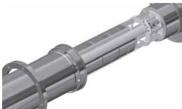
Fig. 28 Pulling out the pump
