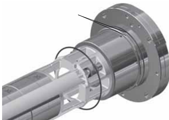
Fig. 29 Replacing the O-rings
