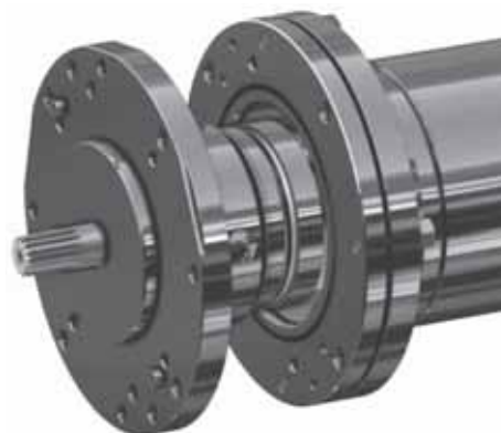
Fig. 23 Mounting the thrust bearing
