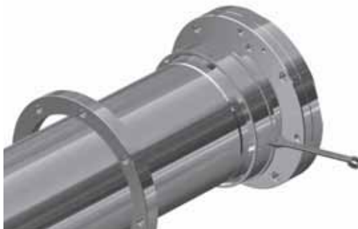
Fig. 27 Separating the pump and sleeve
