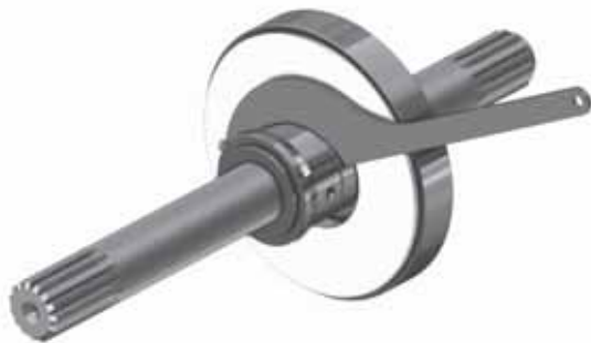
Fig. 18 Loosening the shaft seal
