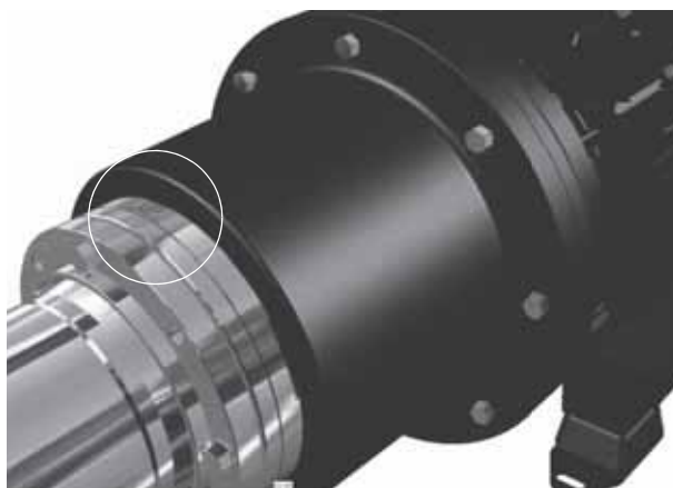
Fig. 35 Correct position of "UP"
