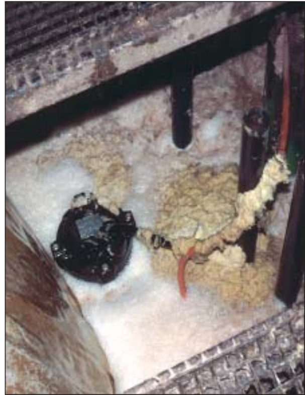
Picture 2 shows one of two Grundfos stainless steel pumps used at a glass wool manufacturing plant for pumping process water with a high content of abrasive particles. Both these pumps are also fitted with the efficient shaft seal flushing system.
