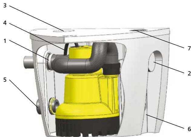
Orifices de raccordement
