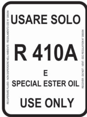
Identification of the refrigerant - External door
