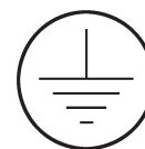
Grounding connection - On the electrical board, adjacent to the connection
