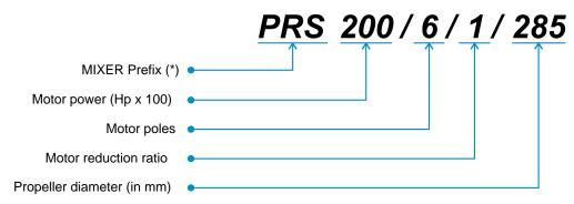
(\*) PRS - cast iron casing - direct transmission
