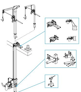
The mixer is supplied as standard with a runner and hoisting hook. All structural work can be supplied in hot-galvanised iron or stainless steel.
