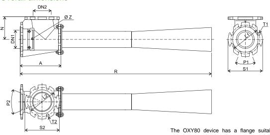
The OXY80 device has a flange suitable for connection to electric pumps having size 80 and 100 delivery ports.
