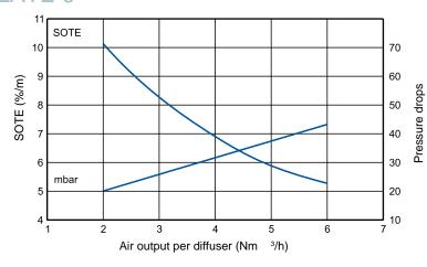
EPDM LP membrane, fine bubbles Oxygen transfer under ATV M209 Density 6.5%
