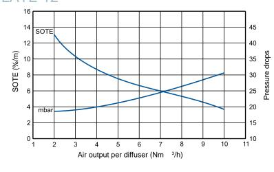
EPDM LP membrane, fine bubbles Oxygen transfer under ATV M209 Density 5.3%
