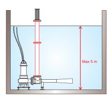
Aspiration pipes for tanks having a depth of 3,5 and 5 mtrs
