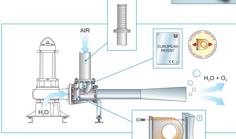
The OXYGEN 80, 100 and 150 ejectors are characterised by the presence of an interchangeable diaphragm covered in corrosion resistant polyurethane material (Vulkollan), which is fixed by two nuts which can be easily replaced and which makes the initial calibration of the system or any maintenance work much easier.
