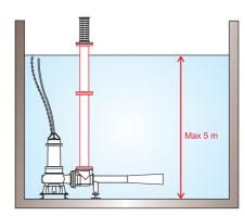
Aspiration pipes for tanks having a depth of 3,5 and 5 mtrs
